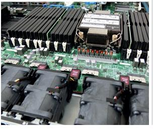
front of the motherboard and flanked on each side by banks of eight DIMM slots. Cable-related clutter is kept to an absolute minimum and all critical components are easily accessible for maintenance and upgrade maneuvers.
