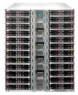
$^2$  32 double precision flops x 28 cores x 2.5 GHz x 144 processors per rack = 323 TFLOPS per rack.
